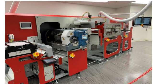
Argonne National Lab, USA. R2R production of Li-ion car batteries.
