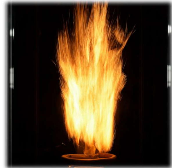
Flame of Iron Powder Eindhoven University of Technology
